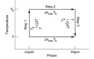
Figure 4. Hypothetical path to calculate  $\Delta h_{vap}$  at a temperature T from data available at  $T_b$  and heat capacity data.
