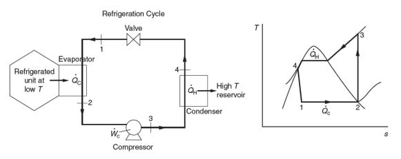
Figure 8. The ideal vapor-compression refrigeration cycle and its corresponding Ts diagram.
