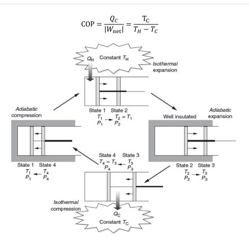
Figure 6. An ideal gas undergoing a Carnot cycle.
