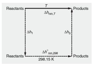
Figure 5. Hypothetical path to calculate  $\Delta h_{rxn}$  at an arbitrary temperature *T*.
