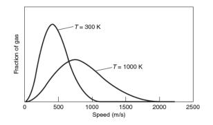
Figure 1. A schematic showing a Maxwell-Boltzmann distribution.
