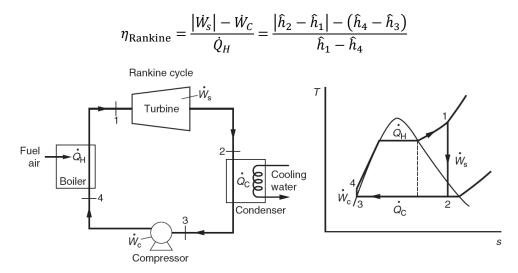
Figure 7. The ideal Rankine cycle and its corresponding Ts diagram.
